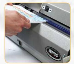
Dual spinning roller insertion for coil diameters up to 15 mm.
